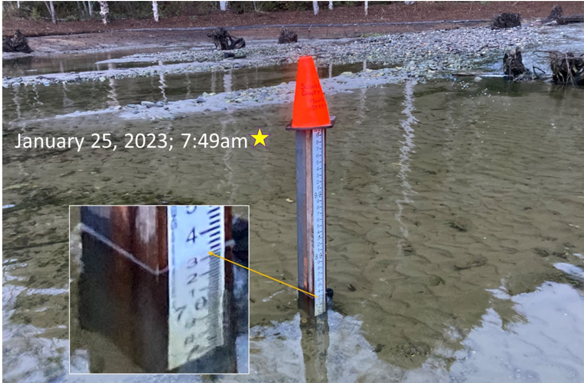
Figure 4. Post-restoration hydrograph placement in the restored embayment located on the upstream side of the new railroad bridge.
