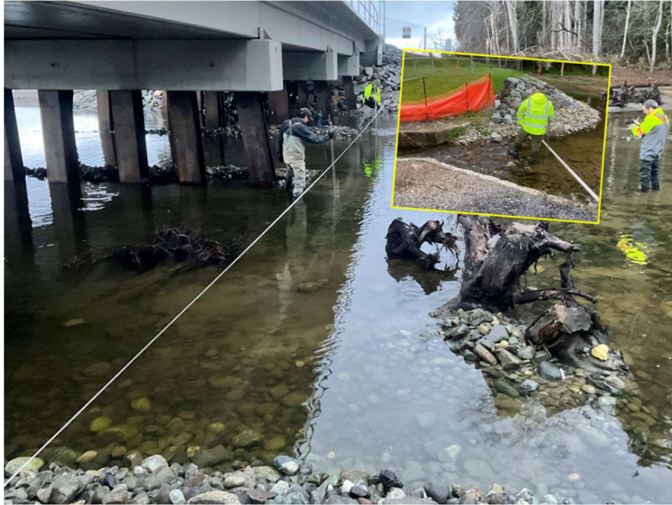
Figure 3. Post-Restoration Velocity Measurement Location at Upstream Margin of Bridge During High Tide with Inset Photo of Pre-Restoration Location
